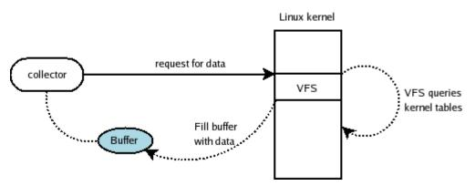
Figure 2 Kernel response to the reading of a file in procfs
