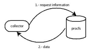
Figure 1 Basic lkmonitor functioning cycle
