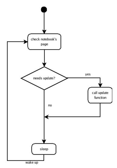
Figure 3 Collector thread behaviour
